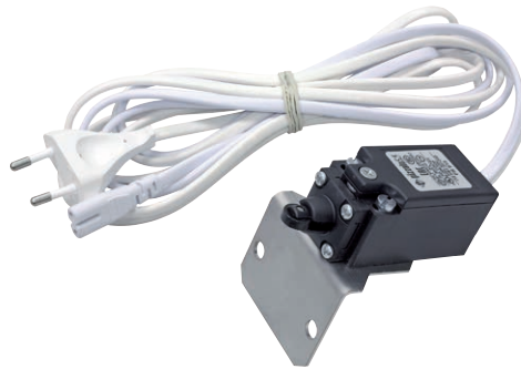
The power supply cable with a door switch that automatically switches on and off the light or other devices when the cabinet opens and closes
