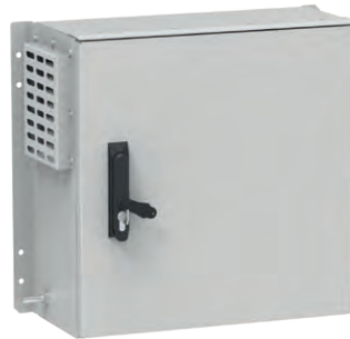
Outdoor cabinet with DIN rails body dimensions 500 x 500 x 210 mm, protection degree IP 55, mechanical resistance IK 10, designed for wall mounting
