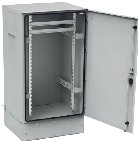
Outdoor cabinet with 19" mounting profiles body dimensions 1140 x 714 x 600 mm, protection degree IP 55, mechanical resistance IK 10, designed in three versions: free-standing (with plinth), wall-mounted or pole-mounted
