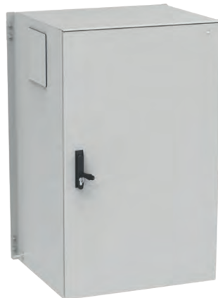
Outdoor cabinet with 19" mounting profiles body dimensions 1140 x 714 x 600 mm, protection degree IP 55, mechanical resistance IK 10, designed in three versions: free-standing (with plinth), wall-mounted or pole-mounted
