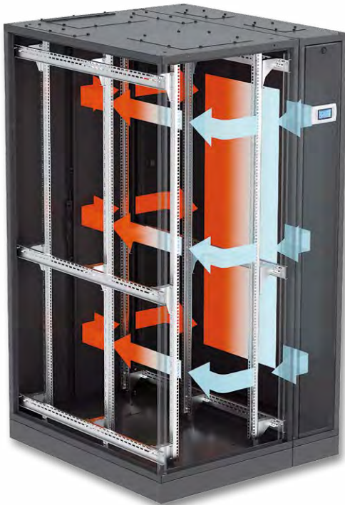
Closed circuit - cooling with side heat exchanger
