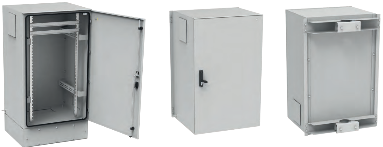
Outdoor cabinet with 19" mounting profiles body dimensions 1140 x 714 x 600 mm, protection degree IP 55, mechanical resistance IK 10, designed in three versions: free-standing (with plinth), wall-mounted or pole-mounted
